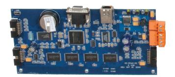
Galaxy is a simple, single platform that allows boards to interact within one cabinet. All 635-series interface boards are "hot-swappable" and intelligent. You can change or add boards while the panel is powered up and operating. And the intelligent design means the boards will synchronize to the system and begin operating within minutes. This provides uninterrupted security during maintenance and upgrades.
