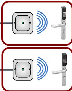
To additional HUBs Up to 16 Locksets (total) per 485 Channel (Any combination of Locksets/Hubs)
