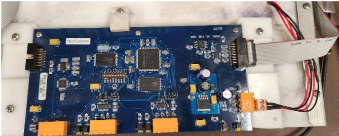
2. Plug in the **12vdc power cable** into DSI Board.
