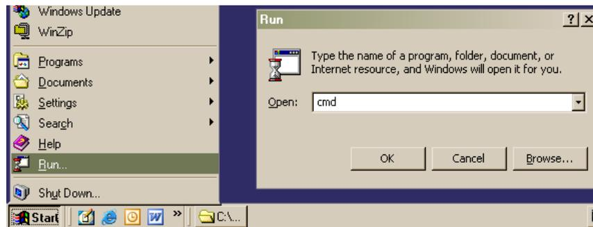
**To ping:** Once the Command Window opens, type the ping command with the target (DVR) IP Address. See figure below. **Syntax is important, so type one space between command and IP Address.** Type "**ping nn.nnn.nnn.nnn**"; where "**n**" stands for the numeric characters in the IP Address
