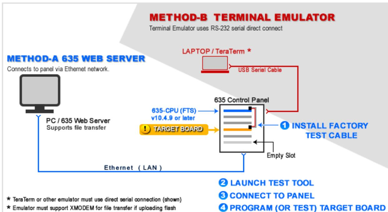
Factory Test Station in field setting - showing both methods (Embedded Web Server vs. Terminal Emulator)
