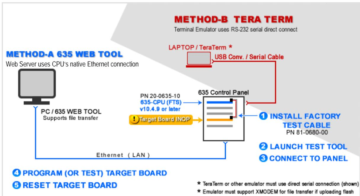
Factory Test Station in field setting - showing both methods (Embedded Web Page or Terminal Emulator).
