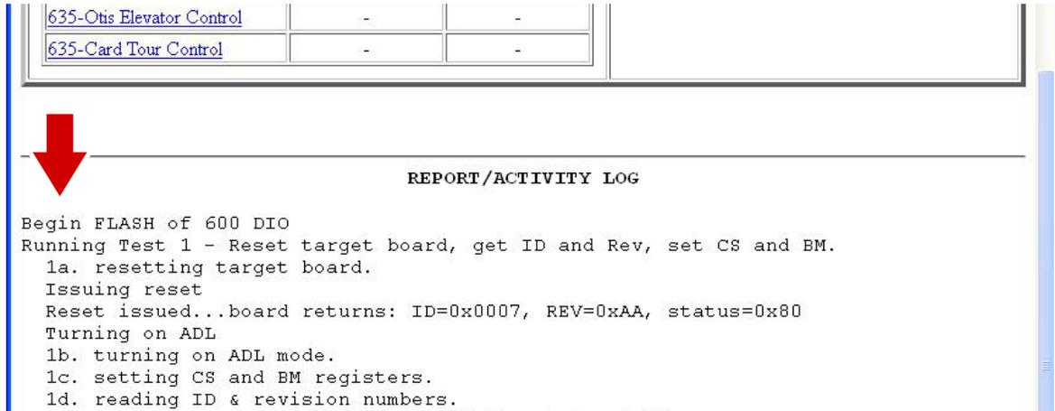
Factory Functions - screenshot showing progress of flashing target board.
