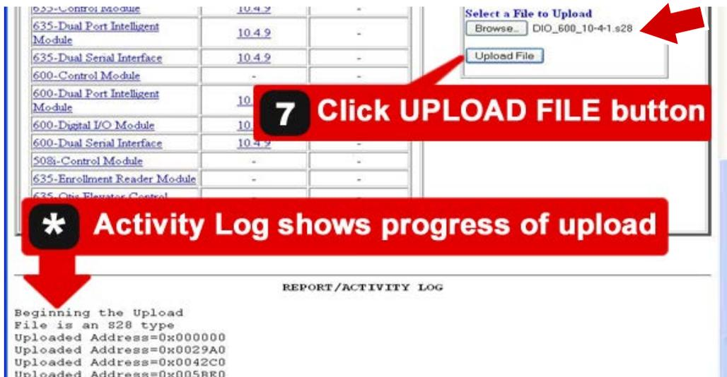
Factory Functions - screenshot showing DIO v10.4.1, but this could be any flash version for any model of board.
