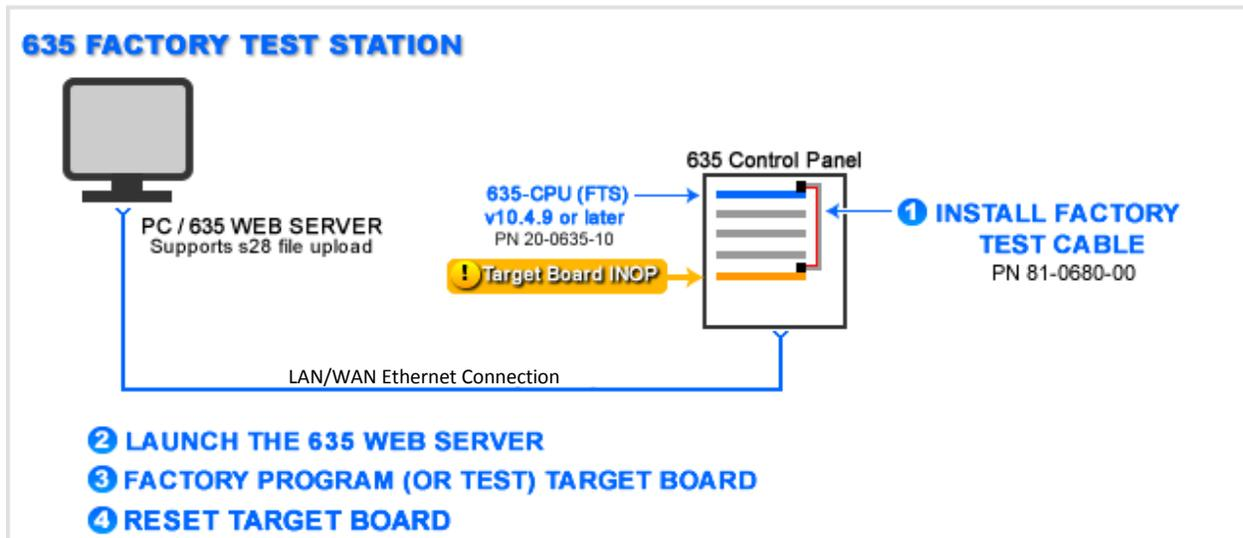
Diagram of Factory Test Station process using embedded 635 Web Server
