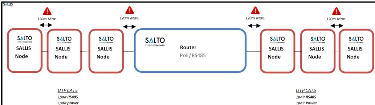
Figure 3-7 Installation example 3 Router PoE
