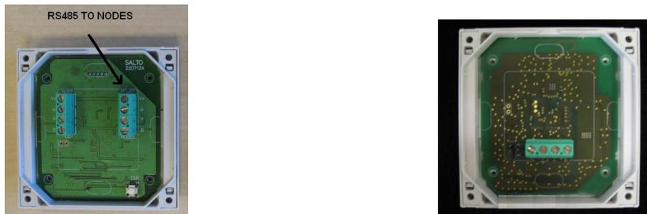
Figure 2-8 Router to Nodes 4-wire connectors
